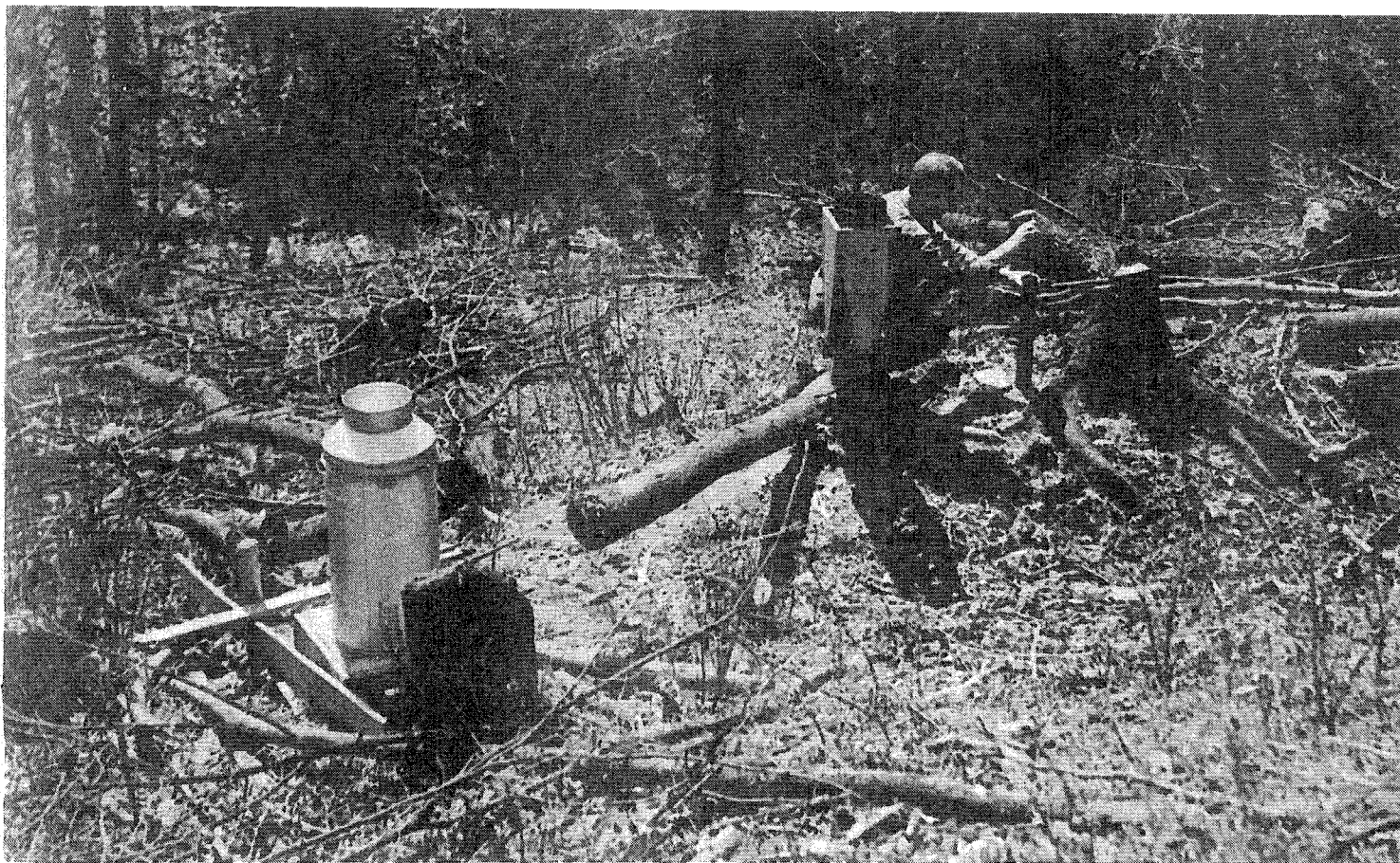
Figure 5.—Recording and standard gages installed in a clearing to measure precipitation.
